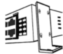
Figure 1. Rack-mount bracket position
